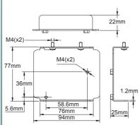
Mounting board for standardized size contactors on thermostat front board. Fits only single pole thermostats versions
