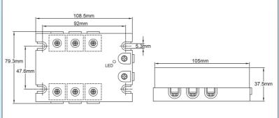
**Dimensions:** 108.5 × 76.3 × 37.5mm Mounting: 4 holes M4, 48 × 92mm spacing Operating voltage range: 24-440VAC, 47 to 63Hz Input signal: 3-32V DC, 12 to 25 mA current
