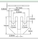
Two ways, 9.3mm pitch, compatible with the BE 2.5mm<sup>2</sup> series.
