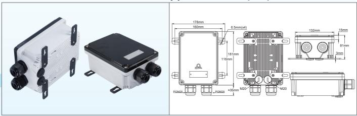
These sealed aluminum boxes are RAL 7015 epoxy painted. They have the same dimensions than the plastic control boxes, and use flat lids. They use the same wall mounting tabs than plastic models. They have been designed for mounting of single or three phase solid state relays of which the cooling is carried by the fins on the rear face.
