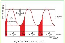
differential. This is the conventional mechanical thermostats operating mode. The successful operation of this mode mainly depends on the temperature sensor correct positioning near the heat source and the compatibility between the heating power and the need of the environment to be heated. The On/Off action does not usually prevent temperature peaks (over-shoot) after switching off the heating, due to the system thermal inertia.
