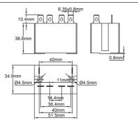
$2\times25A$  250V resistive (AC1) (CE and UL) NO contact, sealed housing,  $6.35\times0.8$  terminals. This relay can be mounted without mounting plate directly on all plastic triggered front provided for bulb and capillary thermostats and electronic controllers, and on the flat fronts of the distribution boxes in this catalog Coil 200-240VAC
