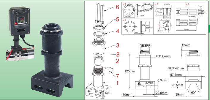
1: Lower part of the foot; 2: Heating cable and temperature sensor sealing gasket; 3: Upper part of the foot; 4: Box gasket; 5: Box locking nut; 6: Bus wires insulator boot; 7: Self locking spring; 8: Self locking spring pin passage 9: Locking blind hole.
