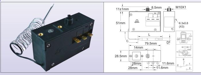
**Housing dimensions:**  $79.5 \times 51 \times 28.5$ mm (6.3 quick connect terminals and manual reset button not included) **Bulb and capillary:** copper or stainless steel depending on temperature range, standard capillary length 1500mm.
