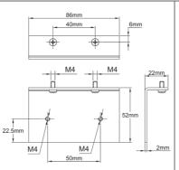
SSR mounting plate on electronic front board. Fits all electronic controllers with SSR output in this catalog Material: aluminum. The kit includes the mounting screws.
