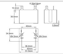
$1\times30A$  250V resistive (AC1) (CE and UL) NO contact, sealed housing,  $6.35\times0.8$  terminals. This relay can be mounted without mounting plate directly on all plastic triggered front provided for bulb and capillary thermostats and electronic controllers, and on the flat fronts of the distribution boxes in this catalog Coil 200-240VAC
