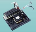
6 relays 16A 250V on thermostat extended front board, with single pole thermostat
