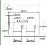
3 ways, 20mm pitch, compatible with the BCA and BCB series.
