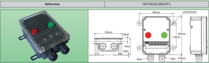
$3 \times 25A$  (AC1), 250V, terminal block with 2 terminals 2.5mm<sup>2</sup> screws and 6 screw terminals 10mm<sup>2</sup>. Red indicator light for power supply and output green light (250V), transparent lid.
