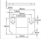
Two ways, 20mm pitch, compatible with the BCA and BCB series.
