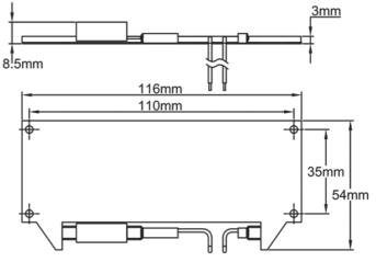
Immediately below the level of the transparent window, the warm air flow it generates prevents from condensation on the window and keeps an optimum ambient temperature for the control devices in the housing. It has a wide aluminum heat exchanger to reduce its surface temperature and a miniature snap-action thermostat limits the temperature inside the cabinet.
