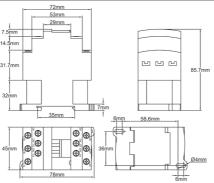
3 × 25A or 3 × 32A 250/400VAC res. (AC1), screw terminals, 240VAC or 400VAC coil. Comply with IEC947-1 (EN60947-1) standard, but its large footprint limits its applications inside control boxes. It does not fit the Y8 types, but can be used in Y6 and Y7 with single pole thermostat.
